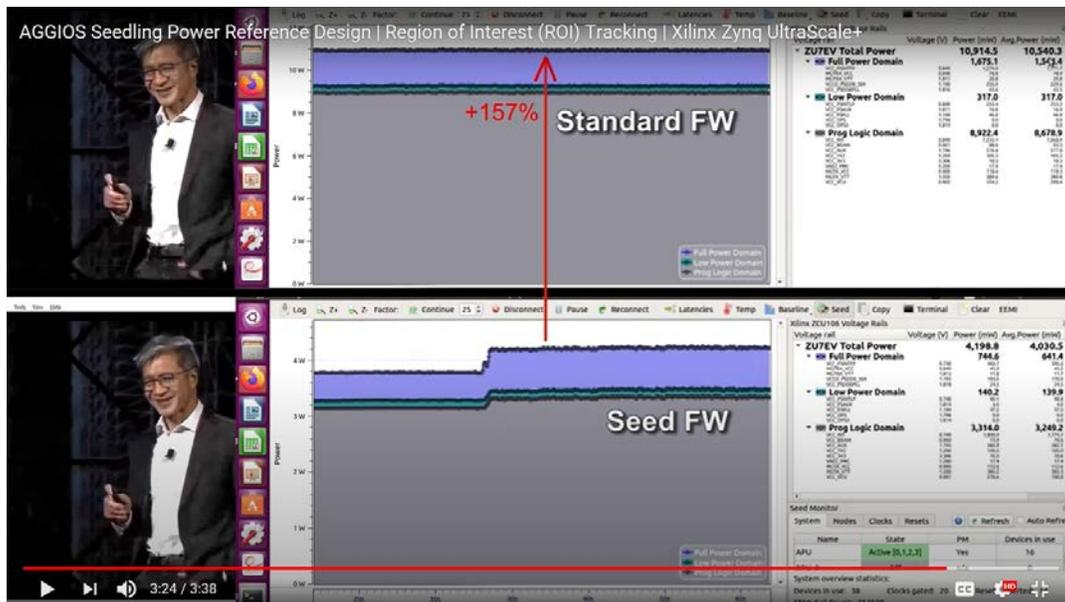
The screenshot above shows the side by side comparison of the original ROI reference design running with the standard firmware in the upper half and the optimized Seedling version below, with power measurements done using the EnergyLab IDE. In this case the penalty for not using the Seed Power Manager is 157%.
