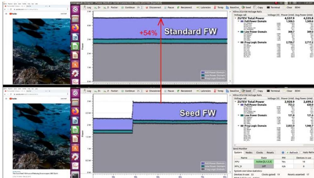
The screenshot above shows the side by side comparison of the VCU reference design running with the standard firmware in the upper half and the Seed firmware below, with power measurements conducted using the EnergyLab IDE. In this case the penalty for not using the Seed Power Manager is a 54% higher power consumption.
